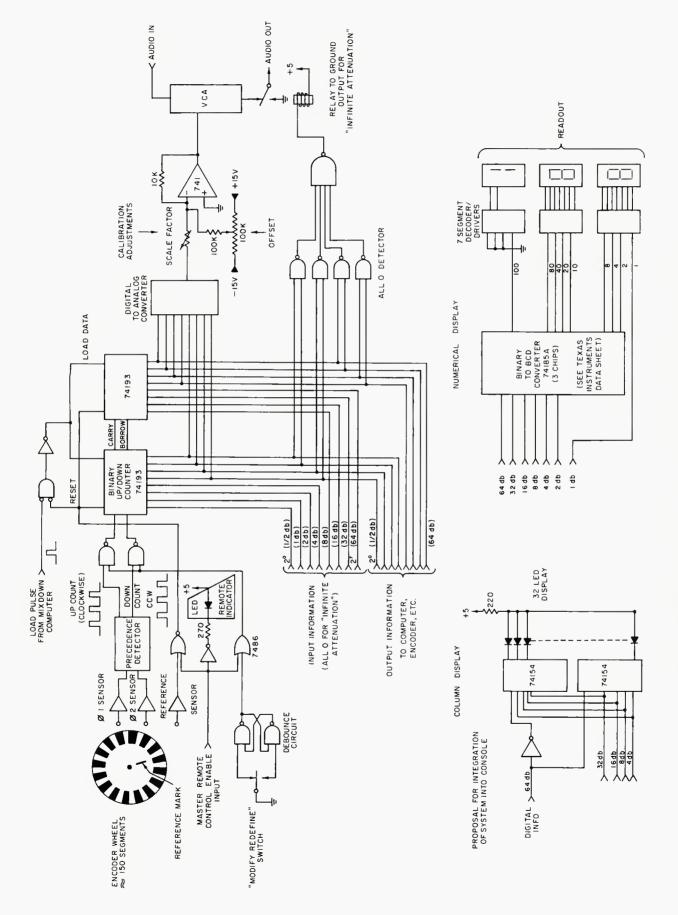
Figure 3. Proposals for the integration of optical encoder systems into a console.
