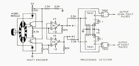
Figure 2. The schematic of a phototransistor amplifier and precedence detector circuit for use with a shaft encoder.
