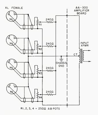
Figure 2. The input mixer section. The transformer feeds the amplifier board input.
