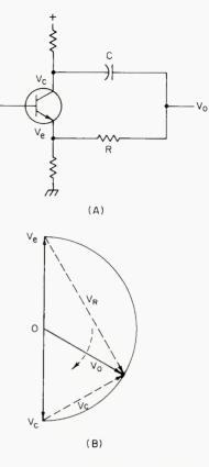
Figure 1. A basic network A), and its vector diagram (B), showing how progressive phase shift, from 0 degrees to 180 degrees, can be achieved without change in amplitude.
