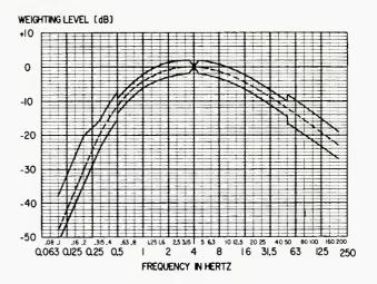
Figure 1. The standard weighting curve.
