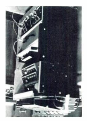
Figure 3. The equipment cabinet. From the top: two AKG C451 battery power supplies; a Sony MX-16 mixer; four Shure M67's; two Shure SE-30 mixers for standby; one more M67; an SAE equalizer; and two of four Bogen power amplifiers.
