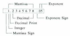
The last two digits on the right end of the display are used for powers of 10 (exponents). To illuminate them, press the Enter Exponent. **EEX** key: To enter the number 35,000,000 in scientific notation, move the decimal point 7 places to the left, and multiply by  $10^{7}$  (3.5 ×  $10^{7}$ ):
