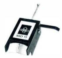
• EMT XSD-15 hand-made stereo moving-coil cartridge is built into its own shell which fits tonearms using the international plug-in configuration. A magnifying lens in the shell simplifies cueing. Each cartridge comes with its own B&K chart showing its frequency response curve from 20 Hz to 20 kHz. FIM distortion, output voltage, and channel separation. Mfr: Gotham Audio (Distributor)
