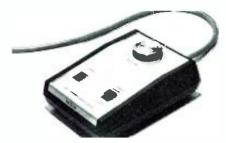
• Increased flexibility in recording speed is made possible with A700 variable pitch control. The device facilitates the continuous sweep variation of tape speed over ±7 musical half tones. Therefore, together with the three standard speeds, the complete range of 2.5 to 5.6 in/sec.; 5 to 11.2 in/sec.; and 10 to 22.5 in/sec can be achieved. A built in sync light indicates "On Speed" at all whole, and fraction of a whole, speed selections. Mfr: Revox Corp.
