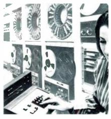
Completely computer-controlled broadcast system 3000 uses the computer as a decision making device as well as for memory. The system can be used for programming, instant reformatting, as well as other applications, such as billing. It automatically provides print-outs of verified logging, has an automatic re-start in case of power failure and a memory storage capability of up to seven days of operation. It has 16 source channels, featuring solid state operation,
