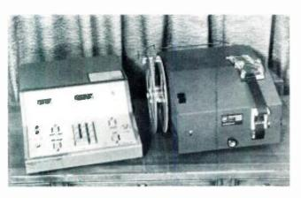
Punch-tape control units provide audio cues for recording on the one-inch show tape.
