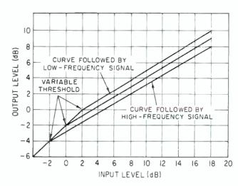
Figure 3. The compression characteristic of a de-esser indicates threshold sensitivity as related to various frequencies.
