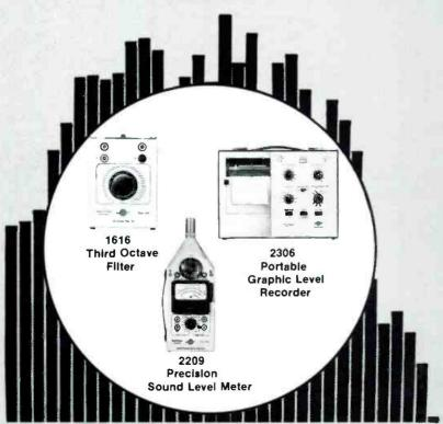
That is why professionals equalize recording studios, auditoria and special masking installations. But the job of equalization must not be left to your ears alone for they are neither calibrated nor qualified for sensing frequency-amplitude unbalance. Therefore, precision acoustic instrumentation must be used.
