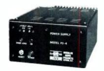
• Adjustable d.c. voltages from ± 14 to  $\pm$  16 V at 4 amps are provided by model 7000 power supply. The unit operates off 115 VAC, 60 Hz input power and includes crowbar overvoltage protection (limiting the output to 18 volts), foldback type current limiting, and inter-locked output protection. Other features include remote sensing, resettable power line circuit breaker, an overload indicator, and front panel voltage adjusting controls. Mfr: Modular Audio Products
