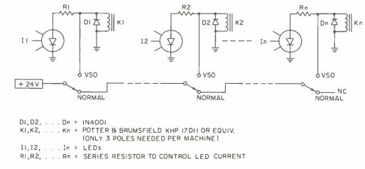
Figure 4. Using this circuit, the capstan motor will run whenever vso operation is selected, regardless of mode.
