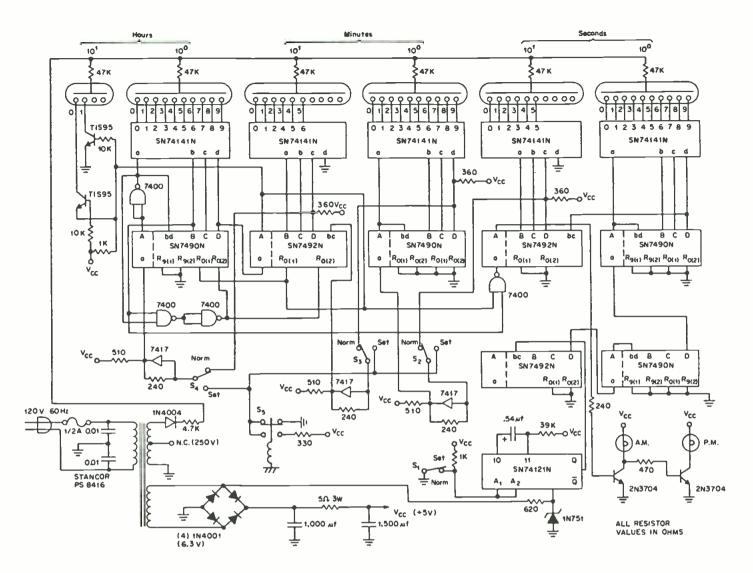
Figure 1. 12-hour clock made up of discrete ttl chips.
