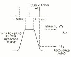
Figure 4. The narrowband filter in the receiver can reduce the output of a wideband system.
