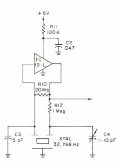
Figure 2. Crystal-controlled oscillator.
