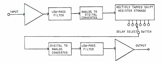
Figure 1. Standard delay line block diagram.
