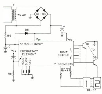
Figure 3. Circuitry of a-kit-built clock.
