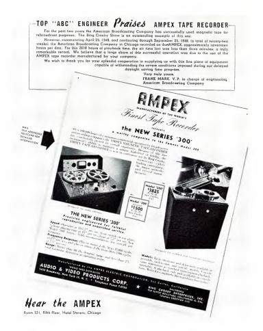
The Ampex 300 appeared in early 1949, running at 15 in./sec. speed (also 7.5) and at both reduced size and price from the 200. This was the first ad. Note the specs.
