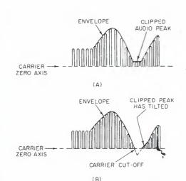
Figure 5. The fiat top of a clipped peak can tilt and overmodulate the a.m. carrier in the negative modulation direction. (Only the upper half of the modulated waveform is shown.)
