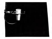
• Almost invisible (3/8 in. diameter. 1/8 in. length) condenser tie clasp microphone CO90 is supplied with a tie bar mount, windscreen, storage pouch and six feet of cable which connects the microphone to its belt clip battery/transformer housing. Optionally, Model CO90E is available powered directly from wireless transmitters. Frequency response is 40 to 15,000 Hz with an output level of -57 dB into a low-impedance input.
