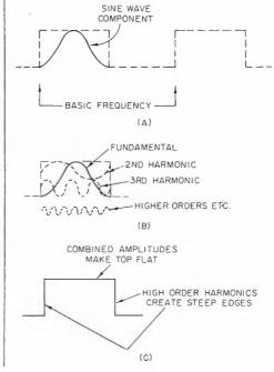
and trailing edges of the pulse. When phasing is correct, then so is the wave-shape of each of these harmonics. All of the amplitudes will combine with the fundamental sine wave to produce a perfectly flat top to the pulse. Since the pulse amplitude does not change during the time of the flat top passage. this flat top represents a d.c. component in the signal.
