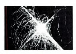
• The Technics by Panasonic people have been demonstrating quad to consumers with a large screen four-channel vectorscope made from a color c.r.t. that has been mis-converged. The resultant display was photographed for us by them to illustrate this special four channel issue.
