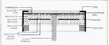
ation in the upper frequency range. The low mass diaphragm means better transient characteristics over the entire frequency range.
