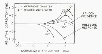
Figure 5. Typical family of free-field correction curves to be applied to a pressure curve.
