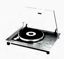
• For kit addicts, the BD1 plinth and cover may be combined with an arm of your choice. The plinth is made of walnut veneer, fitted with spherical, antivibration feet. The cover is acrylic, in bronze, hinged with a two-position stay. The unit stands on a totally enclosed metal base. Dimensions are 15 x 131/4 x 3 ins. Claimed rumble is -65 dB and hum level, -80 dB. BD2/A, an integrated assembly, including tone arm with automatic lift off, is also available, as well as larger units.
