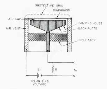
Figure 2. Schematic view of an air-condenser microphone.
