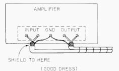
Figure 4. Poor wire dress can create crosstalk problems. (A) Poor dress. (B) Good dress.
