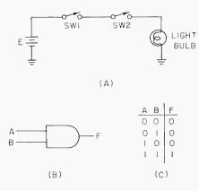
Figure 1. The AND Gate. (A) Circuit diagram. (B) AND Gate logic symbol. (C) Truth table for AND Gate.
