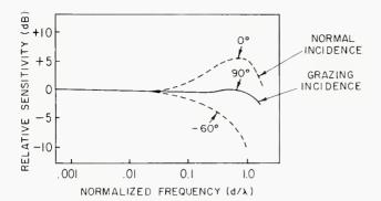
Figure 6. Parallel (ninety degree) incidence and off-axis frequency response characteristics of a typical pressure microphone.
