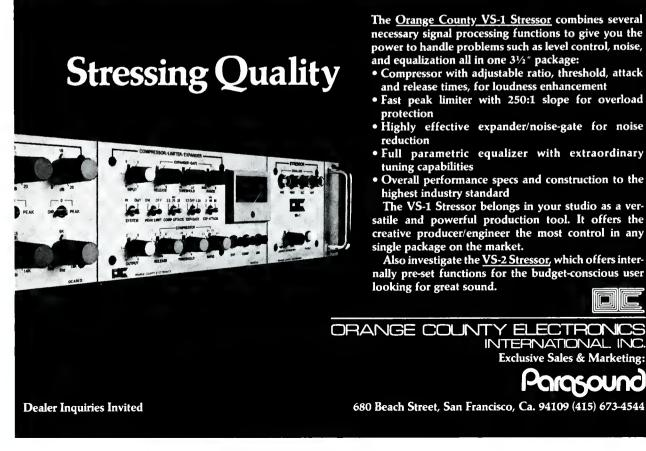
necessary signal processing functions to give you the power to handle problems such as level control, noise, and equalization all in one 31/2" package:
