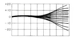
Figure 1. The frequency response of a treble tone control at various settings. Note the shelving shapes, and the fact that the curves are reciprocal: that is, the boost and cut responses are mirror images of each other.
