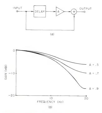
Figure 3. A first-order, non-recursive filter (A) Block diagram. (B) Frequency response.
