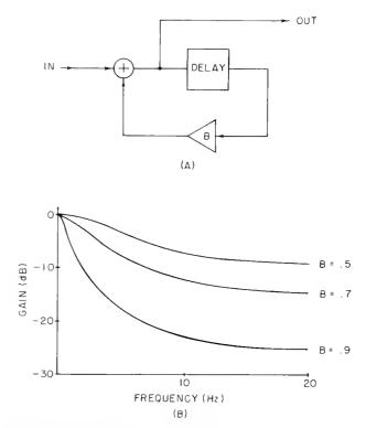
Figure 5. A first-order, recursive filter (A) Block diagram. (B) Frequency response.
