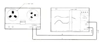
Figure 5. Test set-up for measuring playback response and channel separation.
