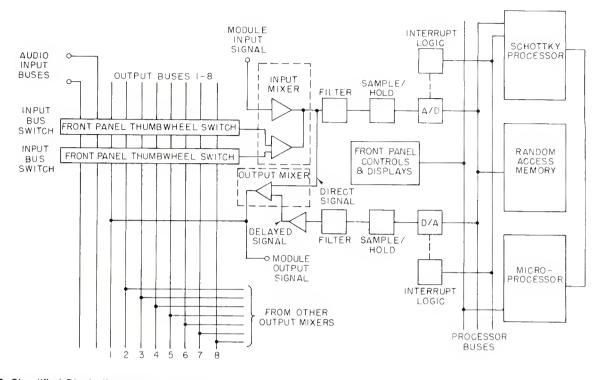
Figure 2. Simplified Block diagram of Shared Access Memory System, showing interface of one module with system.
