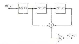
Figure 1. A basic digital low-pass filter.
