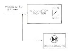
Check the accuracy of the modulation meter with an oscilloscope.
