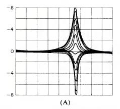
Figure 4. (A) A set of frequency response curves for a constant-Q equalizer with a Q of 3.2. Curves with such a narrow bandwidth tend to cause objectionable coloration when used in the boost mode, and are useful only for special effects, such as telephone filters or simulation of old-time recordings. However, in the cut (or "notch") mode, such curves are useful for filtering
