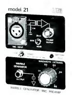
The model 21 Warble Generator/Microphone Preamplifier.
