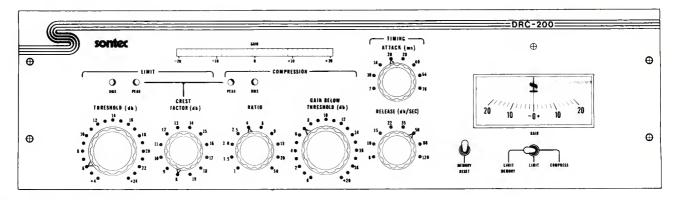
Figure 2. Front Panel Layout
