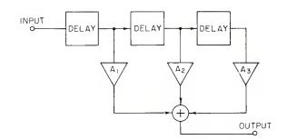
Figure 2. A tapped-delay filter.
