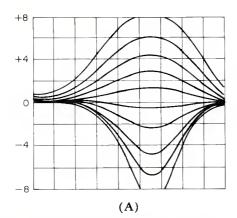
Figure 2. (A) A set of frequency response curves for a constant-Q equalizer with a Q of 0.29. Note that the affected portion of the frequency spectrum is greatest at the maximum-boost position, and continuously decreases as the equalization is moved towards maximum cut. This characteristic tends to produce an equalization effect whose tolerability to the ear remains
