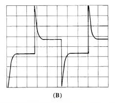
relatively constant as the amount of boost/cut is varied. (B) The equalizer's square-wave output for a 12 dB boost. Note that the very low Q of 0.29 produces a very large overshoot, and that it takes a relatively long time for the overshoot to decay to the final level. However, no ringing is present.
