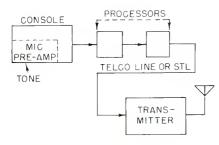
The basic chain is measured. Disable the AGC and other processing units, and make sure that the load on the transmitter is the antenna system.
