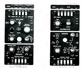
Plug-in modules for the model 200 Mainframe. On the left is the model 2000 Sine Wave Frequency Response Module. Next to it is the model 2010 Level and Frequency Detector.
