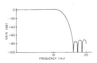
Figure 4. Frequency response of a 32-tap low-pass filter.
