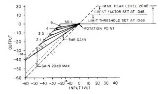
the function led's will remain extinguished. At -15 input level, the rms Compression led will light and will remain lighted as long as the level is above -15 but has not reached the point where any limiting action occurs. At +15 in, the output will be +10.
