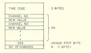
Figure 2. Table format for a single frame. N changes occur within the frame, requiring 2N + 5 bytes. Several tables are packed in one 256-byte record on the disc.
