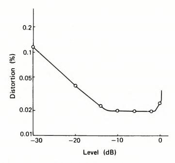
Figure 4(B). Output level distortion characteristics.
