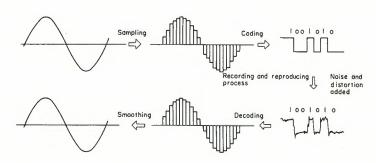
Figure 2. Principle of PCM recording.
