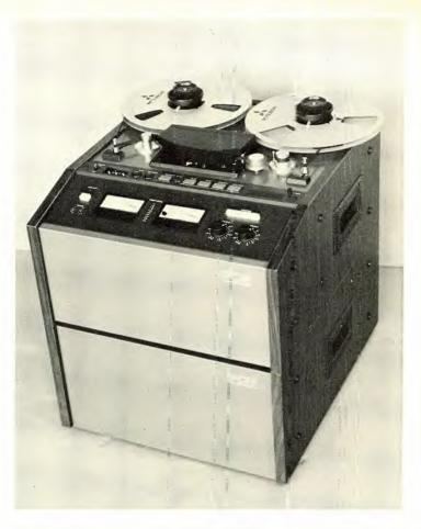
Figure 7. Two channel fixed-head PCM recording deck.
