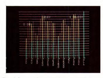
Figure 3. Response of a speaker before room equalization (yellow) and after (green).
