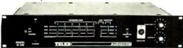
**AUDIOCOM SWITCHBOARD**, portable or rack mount, segregates six external intercom lines into three separate non-interfacing circuits; or stage, lighting and sound crews can communicate independently, jointly, or may be mixed. Contains 24 Vdc power supply with optional, rechargeable battery pack. Smaller power supplies also available.
