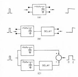
Figure 3. (A) Input and output of a low-pass filter with a very long time constant; (B) A low-pass filter with an extra delay inserted; (C) A - B = C.
