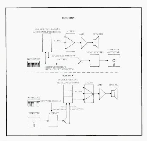
Figure 3. A simplified block diagram showing memory record-
