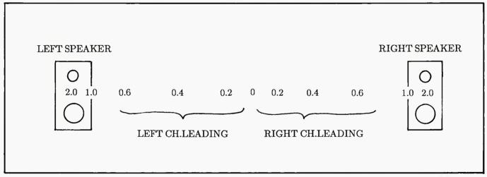
Figure 4. Approximate image location between loudspeakers vs.time difference between channels, in milliseconds. (Listener's perception; listener sitting centered between speakers at a 60-degree listening angle.)
