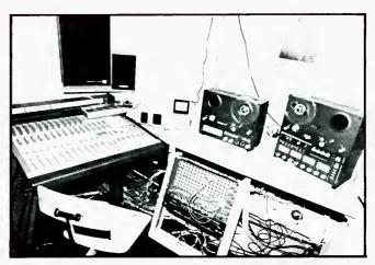
Figure 2. Tascam 22-4 4-track and 22-2 2-track tape decks are side-by-side on a small rack which is housing a patch bay, Lexicon PCM-60, Symetrix compressor/limiter/noise gate/expander, and DeltaLab CompuEffectron.
