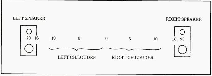
Figure 3. Approximate image location between loudspeakers vs.intensity difference between channels, in dB. (Listener's perception; listener sitting centered between speakers at a 60-degree listening angle.)
