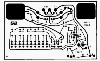
Figure 2. The foil side of the printed circuit board.
