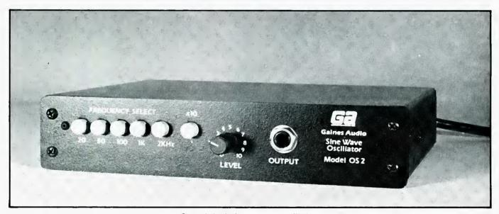
Completed sine wave oscillator.
