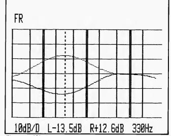
Figure 3(C) Boost and cut range of the low mid control for the equalizer section of the input modules.
