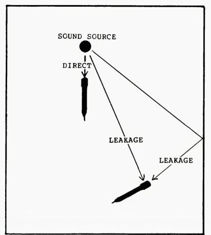
Figure 6. A distant microphone may pick up leakage, also resulting in a distant sound quality.
