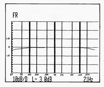
Figure 2.(A) Frequency response to 21 kHz.
