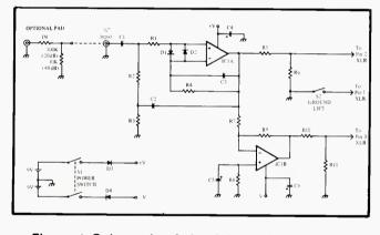
Figure 1. Schematic of circuit for active direct box.
