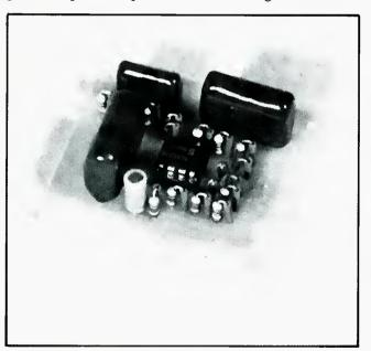
Figure 4. The completed circuit board.
