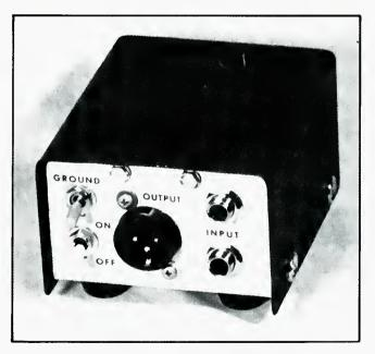
Figure 5. The completed direct box.
