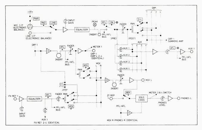
Figure 1. Signal flow diagram.
