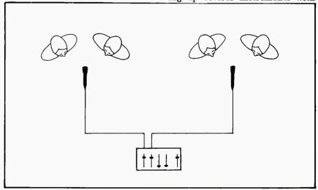
Figure 3. Multiple mic'ing with several sources on each microphone.
