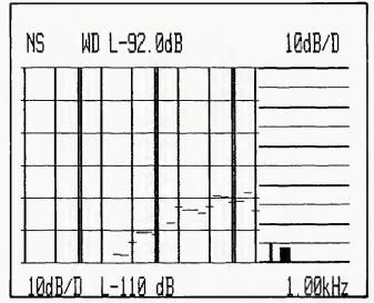
Figure 4. A-weighted signal-to-noise ratio analysis.
