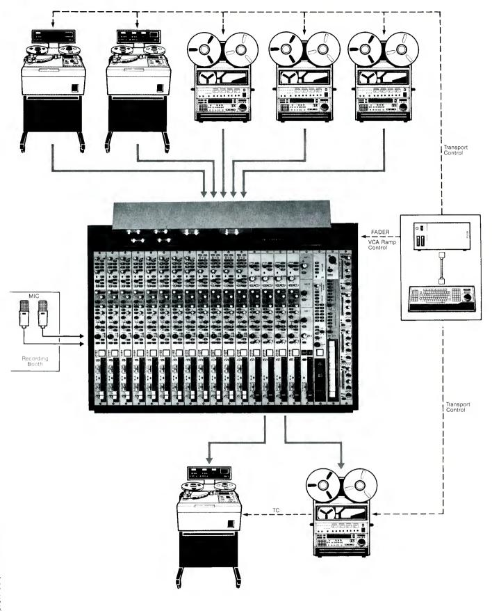
Figure 3. A typical video post production setup, using the MXP-2016 console.
