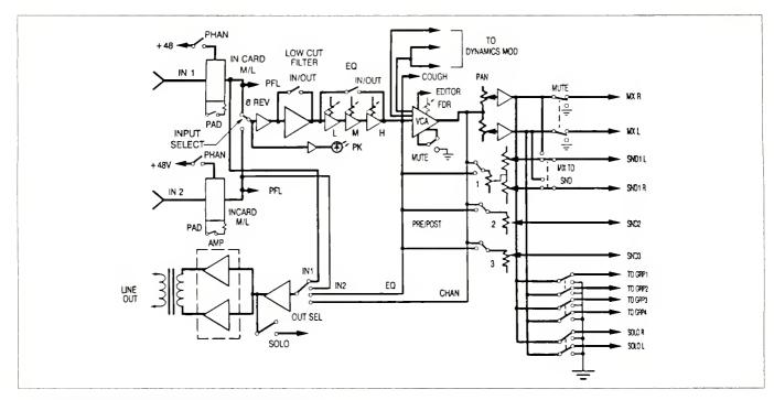
Figure 1. A block diagram of the MXP-2016 signal routing.
