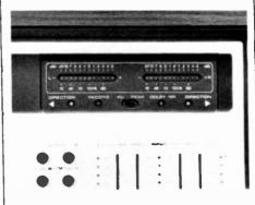
The recording level is indicated by a light bar consisting of twelve light emitting diodes which are calibrated from —20 to +5 dB. The LED's ballistics can be set for either VU (average) reading or for peak reading by using the VU/PEAK switch centered below the meters.
