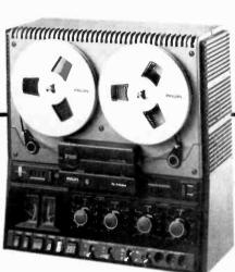
Philips N 4504 is a three-head, three-motor tape recorder which sells for \$450. Its signal-to-noise spec is 60 dB or better at  $7\frac{1}{2}$  and  $3\frac{3}{4}$  ips. It accommodates 7-Inch reels. Circle Reader Service No. 84.
