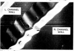
Mistracking Damage A Commercial Recording After Just One Play With Top-of-the-Line Name Brand Cartridge at 10 Gram Tracking Force Mistracking — Critical Damage
