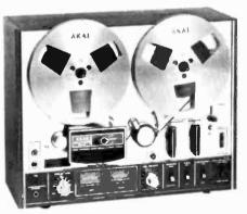
Akai's 4000DS Mk II accommodates 7-inch reels and also offers a choice of T\(^1\)2 or 3\(^1\)4 ips tape speed. It has a 3-head system which includes a one-micron-gap playback head. \$350. Circle Number 62.
