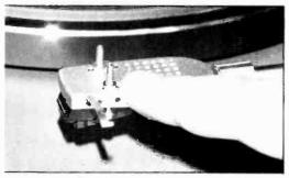
If your pickup carrier permits, install the mounting screws with the nuts on top (on the outside). This makes it easier to make a precise stylus overhang adjustment.
