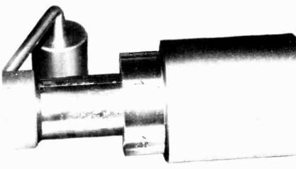
If your tonearm won't balance, even with the counterweight jammed almost against its stop, check to find the small accessory weight which is often provided to add to the back end of the tonearm.
