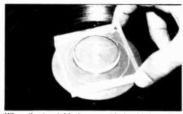
When the turntable is assembled, with its locking screws released, check for 360° balance with a gauge like the Audio Kare AK-5. or a floating platter, adjust the support screws; adjust the feet, using tape shims, if necessary.
