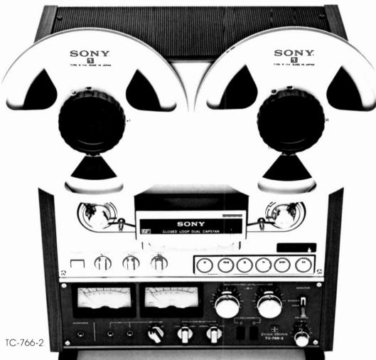
AN INCREDIBLE 0.018% (WRMS) AT 15 IPS, AND 0.04% (WRMS) AT 7½ IPS. Closed Loop Dual Capstan Tape Drive System. One capstan extends from the motor shaft itself, eliminating intervening gears that can hamper speed accuracy. The other tape drive capstan connects through an extremely steady belt-drive inertia flywheel.
