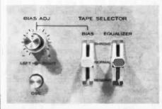
Pressing the OSC button automatically disconnects the input signal and applies the blas test tones alternately to the tape. Left and right blas level are individually adjusted through concentric controls.
