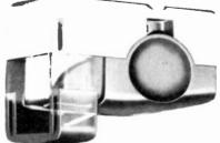
est diamond stylus with the smallest cantilever of any production cartridge known. For example, the cantilever of the TK7SU is just 0.5 mm in diameter at the large end of the hollow tube, tapering to just accommodate the 0.11 mm diamond at the tip. The squareshank stylus can be precisely oriented
