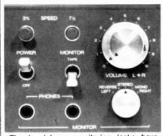
The headphone monitoring jacks have individual left and right level adjustments and a selector that permits stereo or mono monitoring, or monitoring of the individual left or right tracks.
