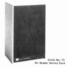
4311 has a 12-inch woofer, a five-inch midrange and a 1.4-inch tweeter in a textured grey or oiled walnut enclosure. Specifications: Power capacity 75 watts RMS continuous power; frequency response, 45 to 15,000 Hz ± 3 dB; distortion, less than 1% third harmonic generation from 100 to 15,000 Hz; sensitivity, 91 dB, 1 watt, 1 meter and 42 dB, 1 mW, 30 feet.
