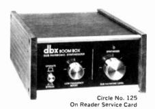
table rumble, acoustic feedback and side effects of warped discs. There are two controls: a sub-harmonic level control which regulates the amount of synthesized signal added to the program; also a low frequency boost knob which is a tone control specially contoured to produce a smooth blend of the synthesized notes into the music. There's also a bypass switch, and a red LED which indicates when the unit is synthesizing. Nationally advertised value: \$199.
