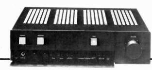
Yamaha's A-1 integrated amp has a DISC switch which is able to electrically direct-couple the phono pickup to the output power amplifier. Direct-current equalizer improves transient response. \$595. Circle Number 101.
