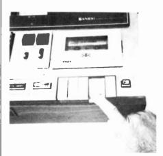
• To demagnetize, simply place the HD-01 in the recorder and hold down the play or start button for about one second. When the LED in the center of the cassette lights, demagnetization has been completed. Circle Reader Service Number 107.
