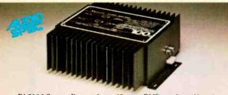
PA610) Stereo Power Amp. 50 watts RMS per channel into 4 ohms, 20-20,000Hz, with no more than 0.05% total harmonic distortion. 3149.95†
