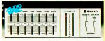
EQZ6200 Graphic Equalizer. 7 traquency bands with 12dB poost or cut. LED signal level meters. Audio muting & equalizer defeat. \$65,95†
