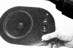
At left is an ordinary 6-by-9-inch car speaker typical of those supplied with cardealer-installed sound systems. At right is the Epicure LS70, one of the two loudspeakers we worked with. The LS70 has a separate woofer and tweeter. Larger than the ordinary 6x9 speaker, mounting holes correspond to those of the 6x9.
