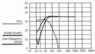
Improved bass response as the result of the low frequency driver and vent working together
