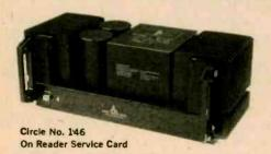
DESCRIPTION: A stereo power amplifier which is FTC-rated at 75 watts RMS per channel into 8 ohms, 20 to 20,000 Hz, at a distortion no higher than 0.01% THD. This unit can be used as an independent power amplifier, or it may be docked with a preamplifier to form an integrated amplifier. It also may be docked with a tuner/preamplifier to form an integrated receiver. The DA-A7DC has its own power and speaker selection switches whose functions can be transferred through
