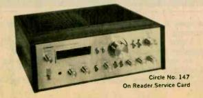
DESCRIPTION: An integrated stereo amplifier, which is FTC-rated at 80 watts RMS per channel into 8 ohms, 10 to 20,000 Hz, at a distortion of 0.005% THD. Features include: switch-selected cartridge resistive loading of 100, 10k, 25k, 50k and 100k ohms and capacitive loading of 100, 200, 300, 400 and 500 pF; a phono input radio frequency interference filter; 12-step left and right output power fluorescent light-bar displays
