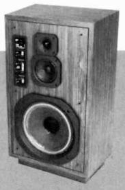
Avid offers the Model 230 speaker as part of its "Un-boxed" speaker line. Designed to minimize cabinet diffraction effects, its drivers include a 10-inch woofer with foam surround, a 4½-inch midrange, and a 1-inch fabric dome tweeter. Crossover points at 475 and 4,000 Hz. Min. recommended power is 15 watts, max. power is 150 watts. Price about \$225 ea. R. S. No. 132.
