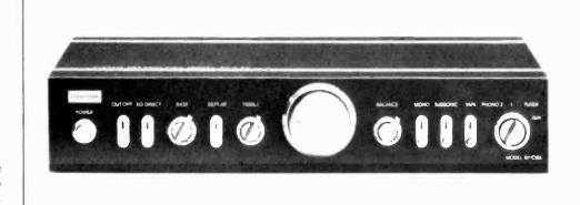
Toshiba's C-15 DC stereo preamplifier has high-gain dual FET DC amplifiers. The phono preamp circuitry is said to handle up to 300 mV without overload for highoutput cartridges and direct-cut discs. The unit has an EQ-Direct switch that allows bypassing the tone controls when used with an equalizer. The C-15 is 10.1 in. wide, 2.1 in. high and 8.2 in. deep. Price: \$300; with black finish (shown) \$310. Circle 99.
