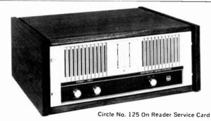
**DESCRIPTION:** A stereo power amplifier FTC-rated for 8 ohms at 220 watts RMS per channel, 20 to 20,000 Hz, at no more than 0.08% THD, or 700 watts RMS monophonic at no more than 0.12% THD.
