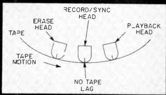
Figure 2. On a multitrack recorder the record head is used as a playback head so that the monitored track is synchronized with the track that is being recorded on. This is called synch.
