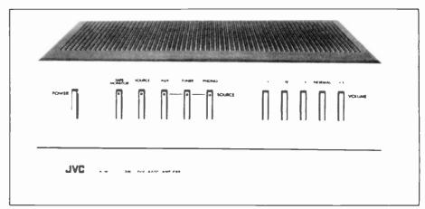
The JVC A-M1 micro power amplifier delivers 50 watts-per-channel RMS into an eightohm load. The total harmonic distortion is 0.03% with a frequency response from 20 to 20,000 Hz. It features a push-button volume control with five levels. This is done because the primary volume controlling would be on the preamp. Price: \$600. Circle 74.
