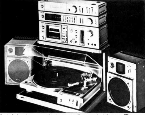
Sony's Avatar micro component systems come with a tuner, turntable, preamplifier and a pair of combination speaker/amplifiers. The GG-20F (\$1,795) is capable of 55 watts-per-channel output with 0.2% THD. The GG-10F (\$1,295) has 20 watts-perchannel with 0.25% THD. Optional cassette deck (\$550). Circle 94 for information.
