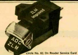
**DESCRIPTION:** A magnetic pickup with a special elliptical stylus and an integral stylus guard. Rated for a 1-gram ±0.25 gram VTF. Recommended output capacity load is 275 pF.
