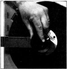
Left • Five pushbuttons control the operation. Small indicators above the switches show the operating mode and whether the tonearm has stabilized and is operating tangent to the record. Right • A rotating pad at the end of a swing-arm presses the record against the platter to help maintain a steady operation.
