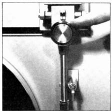
• The tonearm hangs down from a pivot. An unbalancing force, which is dialed in directly, causes the tonearm to move towards the record and apply the tracking force. The stylus force range is 0 to 2.5 grams in 1 gram increments,
