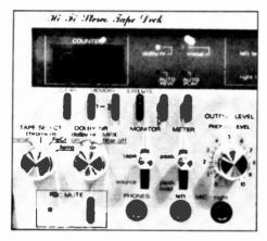
metal-capable cassette deck. Basically, the machine has the appearance and features of cassette decks that originate in the Far East, where the new Philips is manufactured. It is front loading with a dual capstan drive, has a three-head system for simultaneous record and playback and a dual-Dolby with selectable mpx filtering, includes microphone and line input mixing with a separate master gain control, and accommodates ferric, ferrichrome-bias, chrome-bias, and metal tapes.
