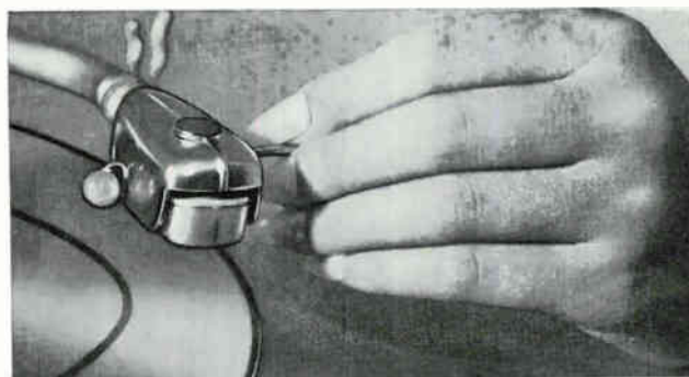
Radiation, emanating from the ball-shaped "Atomic Jewel" clipped to the pickup, separates disc from dust.
