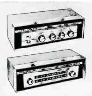
Mates" are a handsomely styled separate amplifier and AM-FM tuner, which offer much value for little money. The tuner features the original Armstrong circuit and automatic frequency control, which "locks in" on FM stations and holds them "in tune." At a price of \$67.50 (Continued on page 22)
