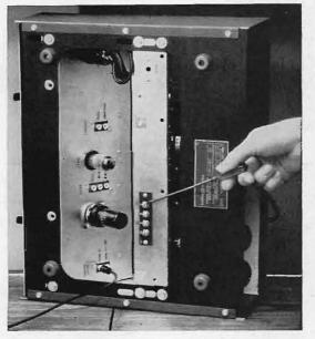
Access to output, input and loudspeaker connections necessitate turning PA-20 on its side. Hum level control is visible.
