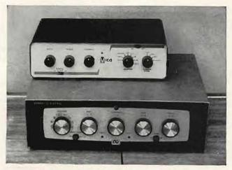
Transistorized Vico 77 is a smaller package than GE PA-20. Latter, however, has more flexibility using vacuum tubes.
