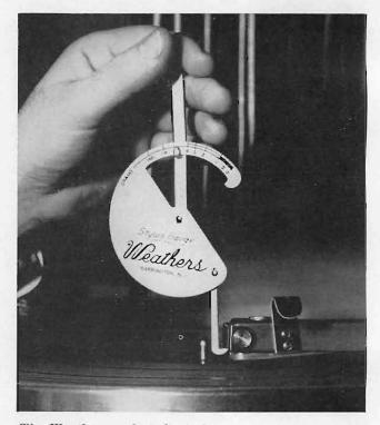
The Weathers scale is basically a counterbalanced lever while the Clarkstan stylus pressure gage works by deflecting a spring.
