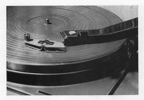
The Audak stylus pressure scale operates like a chemist's balance, employing calibrated weights.
