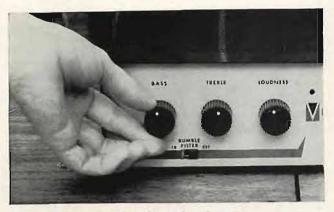
Bass control does boost, but does not cut. Loudness control also means volume adjustment in the Vico Model 77.
