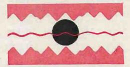
Top view of groove tracing by conventional stylus shows a case of putting a round peg into a ditch made by a square culter. Unable to follow the contour, the stylus is "pinched" upward.
