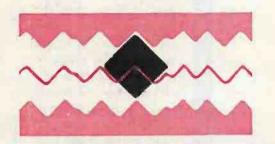
Square contour allows pyramid point to trace accurately even extreme modulations incised into the groove. The distorting vertical motion of the "pinch effect" is thereby eliminated.
