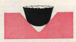
Conventional rounded stylus touches groove only tangentially at two points, resulting in enormous contact pressures. Even a lightweight pickup exerts point pressure of many tons per square inch.
