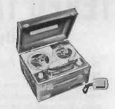
permits the use of a larger external loudspeaker. A neon bulb indicates the recording level and a crystal microphone comes with the unit. Dimensions:  $11\frac{3}{4} \times 9\frac{7}{8} \times 7\frac{1}{8}$ inches. Price: \$54.50. (Lafayette Radio, 165 Liberty Ave., Jamaica 33, N. Y.)
