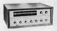
FM sensitivity is 3.5 uv for 30 db quieting (2.5 uv for 20 db), the bandwidth is 240 kc at the 6 db points, the circuit features AFC, a Foster-Seeley discriminator
