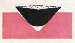
Pyramidal point, resting on broader areas of the groove wall widely distributes stylus weight, avoiding excessive contact pressures, reducing frictional heat and mechanical wear.
