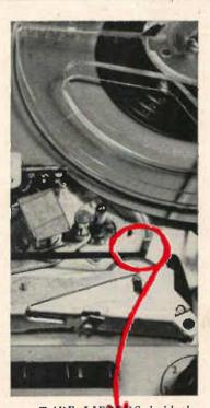
TAPE LIFTUS hold the tape away from the head surfaces during rewind and fast forward. The Tandberg Model 6 employs this type of mechanism.
