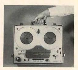
THREE.MOTOR DRIVE is one possible indication of quality in the transport mechanism. In the Knight KN-4000 tape player, the capstan and each of the two reels are driven by separate motors.
