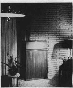
The Klipschorn is a classic instance of a folded-horn design, using a corner of the room as an extension of its horn.
