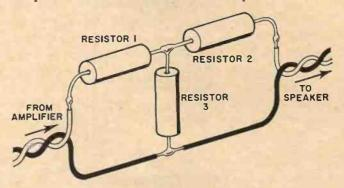
Figure 6. Resistance network in speaker line may be necessary to keep main speakers from sounding louder than extensions at a given volume setting. Resistors 1 and 2 should be 0.3, and resistor 3, 0.8, of the main speaker's impedance.
