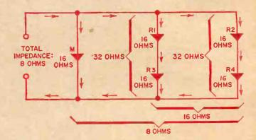
Figure 3. Sketch for a system with 16-ohm main speaker (M) and four 16-ohm extensions (R<sub>1</sub>-R<sub>1</sub>) arranged in series-parallel to provide a total impedance of 8 ohms.
