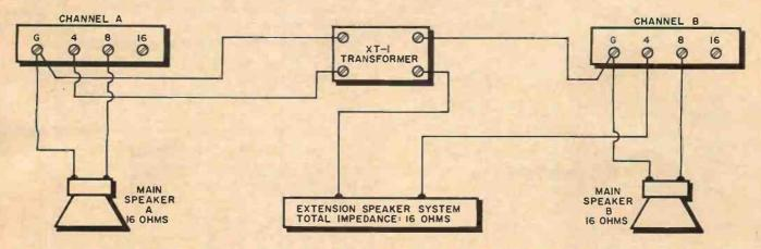
Figure 4. Wiring plan for obtaining a blended mono signal for extension speakers by the incorporation of an Electro-Voice XT-1 mixing transformer. This device maintains stereo separation on main speakers while providing mono output for extension speaker use.
