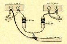
resistors to blend the two stereo outputs and feed these to a separate amplifier to drive the remote speaker. If your amplifier has a third-channel output, use this to feed the separate amp. Otherwise, use the network shown above. The separate amplifier should have its own input level-set control, to allow you to cut down its input signal if necessary to avoid overloading it.
