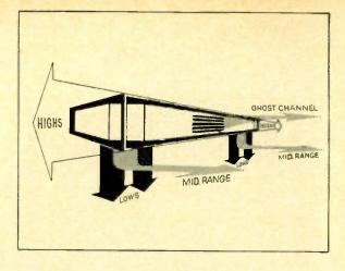
directed downward and outward through openings in the bottom of SONORAMA. High frequencies emanate from super-tweeters that are angularly placed at each corner. Bass frequencies take two directions, both downward through their own diaphragms, and through a third "ghost" channel inside SONORAMA and then out the center. Thus, SONORAMA sends out a full 180° "curtain of sound" that fills every corner of a room!
