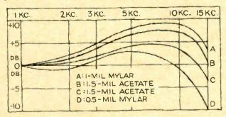
tape. Four of the response curves, representing upper and lower limits as well as typical intermediate responses, are shown in the graph above.
