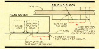
to leave a visible mark across the tape. By hand, shuttle the marked spot across the head until it corresponds to an audible "plop." Hold the tape in that position, and use a marking pencil to indicate any convenient spot to one side of the head. The distance from that mark to the magnetized needle's mark is the displacement distance, and should be marked permanently on your splicing block.
