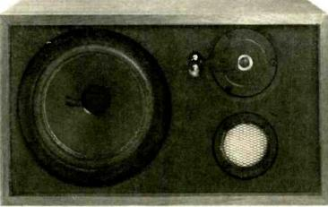
The AR-2 series of speaker systems made by Acoustic Research has long been considered a standard of high-fidelity performance where cost requirements made technical compromise necessary. The best speaker system in the series, the AR-2a<sup>×</sup>, was the result of a series of refinements of the original AR-2. The most important such change has probably been the conversion of the older unit to a three-way system.
