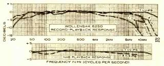
The  $7\frac{12}{2}$  and  $3\frac{34}{2}$ -ips curves show the recorder's response to both the 111 and 202 tapes with the appropriate equalization-switch settings. Although frequency responses are identical at the two speeds, signal-to-noise ratios should be better for the 202 tape.
