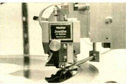
The Westrex stereo cutter head looks rather ponderous to audiophiles accustomed to the light appearance of phono cartridges. The tube whose flattened end is adjacent to the cutting stylus is connected to a vacuum pump that draws off the material (called "chip") cut out of the blank acetate surface to form the groove. The "tone arm" that carries the cutter head is the entire massive, elbow-shaped section resting on the lathe hed in the photo above. (All photos by the author.)
