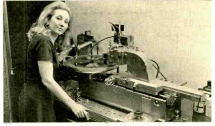
The Scully master-disc cutting lathe operates under the control of engineer Gladys Hopkowitz. Note the built-in groove-inspection microscope on its swivel arm. The precision machining of the lathe—and the massive construction needed to maintain that precision—have to be seen to be appreciated.
