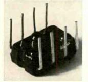
Ultra-reliable Integrated Circuits: Seven IC's are included in the 387 . . . totalling 91 transistors, 28 diodes, and 109 resistors.
