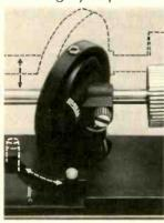
Mode Selector of Dual 1219 lowers tonearm base for single play. Stylus tracks at correct 15° angle.
