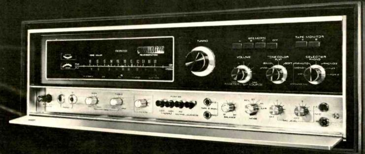
And if you want to get down to the nity gritty, the EX-9000 has an FET front end with sensitivity at 1.6 microvolts to bring in the most tain the afted stations. There are 4 IC's in the IF combined with a 1dB capture ratio and 40dB selectivity, you can pin-
