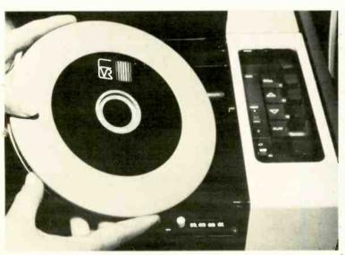
The round EVR cartridge (shown above being loaded into the CBS player) contains special film meant for photo-electric scanning. SelectaVision, still under development by RCA, employs laser scanning of a holographic image embossed on a clear vinyl film.
