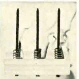
New solderless connection techniques: Tension-wrapped terminal connections plus plug-in circuit modules result in the kind of reliability associated with aerospace applications.
