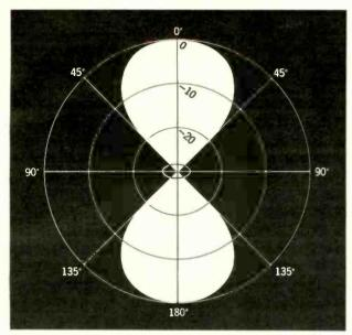
Fig. 1(b). A bidirectional microphone responds to sounds coming from directly in front or behind, but not from either side. The concentric circles are arbitrarily calibrated in output levels.
