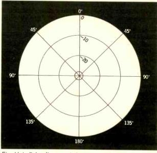
Fig. 1(a). Polar diagram of the ideal non-directional response of an omnidirectional microphone. The microphone, symbolized in the center, is equally sensitive to sounds from any direction.
