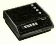
TEAC has added a moderately priced stereo cassette deck to its line of cassette equipment. The Model A-23 has a frequency response of 60 to 10,000 Hz ±3 dB, and a signal-to-noise ratio of 43 dB. Wow and flutter are under 0.23 per cent. The deck's controls include separate rotary knobs for each channel to adjust recording and playback levels, six push keys (record, play, stop-eject, fast-forward, rewind, and pause), and an on/off push-
