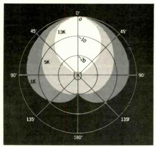
Fig. 1(c). A unidirectional (cardioid) microphone is intended to be aimed at the desired sound source. As with other types, its angle of acceptance narrows as the sound frequency increases.
