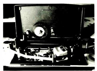
The head cover on the Akai GX-365D is hinged, permitting easy access for inspection and maintenance. A special capstan sleeve and pinch roller for 15-ips operation are stored on its underside.
