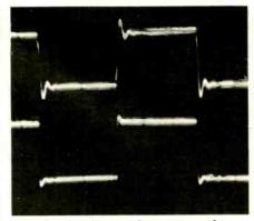
(7) DC-300 input and output waveforms
