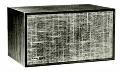
● A NEW member has been added to the Dynaco speaker family. The Model A-10, a very compact two-way system, closely matches the acoustic characteristics of the larger Dynaco A-25 and A-50 speakers. The A-10 uses the same soft-dome tweeter as the A-25, and its 6-inch woofer has the same magnet structure used on the 10-inch woofers of the A-25 and A-50. The 6-dB-per-octave crossover is at 1,500 Hz. Unlike the larger systems, the A-10 has no tweeter-output level adjustment.
