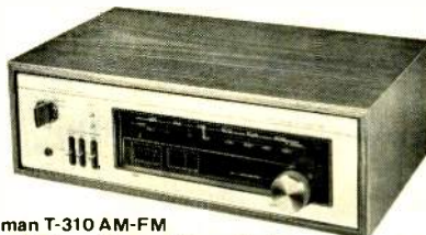
Luxman T-310 AM-FM Dolby Stereo Tuner IHF sensitivity 1.7 uv Selectivity 75dB, Capture ratio 1.5dB Total harmonic distortion: 0.1% @ 400 Hz, mono, 0.12% @ 400 Hz, stereo. Dolby B-type circuits for decoding FM and tapes, Dolby calibration controls. Switchable/variable AM/FM muting. Dimensions 19 1/8" x 11 1/8" x 6 1/2" Weight 21 lbs $595 00
