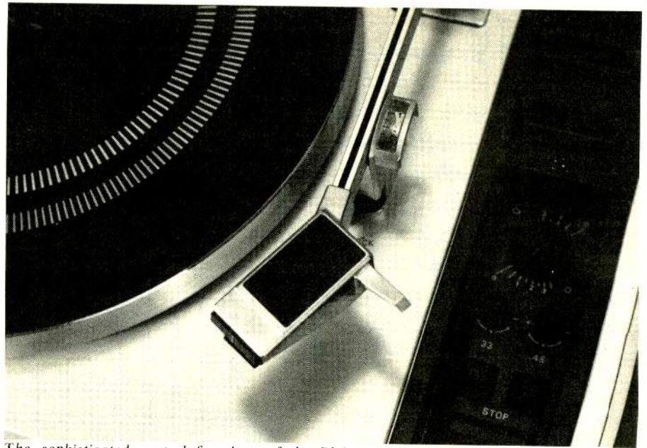
The sophisticated control functions of the Philips 209S-Electronic turntable are shown partly concealed behind the sliding cover. With the cover in place the unit automatically selects proper speed and arm setdown. Note the built-in stylus-force gauge in the arm rest.
