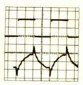
Diagram E: 1. A good conventional speaker with wide, flat frequency response and low distortion still cannot reproduce the original square wave signal.
