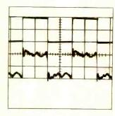
2. Beovox Phase-Link loudspeakers can reproduce square wave accurately by virtually eliminating phase distortion.
