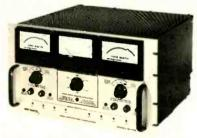
sign with a rated output of 150 watts per channel into any load impedance from 4 to 16 ohms, with a maximum of 0.5 per cent harmonic or intermodulation distortion. Rated power is available at any frequency from 20 to 20,000 Hz, both channels driven simultaneously. The signal-to-noise ratio is 90 dB.
