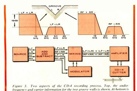
a block diagram of the CD-4 recording chain from tape machine to disc cutter.
