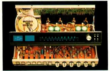
Push-button electronic time-delayed diode switching provides noise-free blends when changing program sources. This innovation allows us to put the controls in the best position for easy operation and the electronics where they can deliver the best performance. Independent tape-to-tape facilities add to the extreme versatility of TR-2075.
