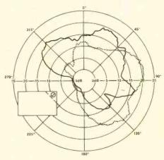
The solid line is the polar characteristic for the Model 301 with the Direct Energy Control set for maximum direct energy and a more intimate sound. The broken line is the polar characteristic with the Control set for maximum reflected energy and a more spacious sound. Fréquency is 8 kHz, bandwidth is  $\frac{1}{3}$  octave.
