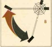
A) Dual's anti-skating system is located within the tonearm system. it applies the necessary counterforce around the pivot and directly opposite to the skating direction. B) The system also provides automatic compensation for the inherent change in skating force that occurs as the stylus moves toward the record center.
