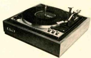
• GARRARD's new Model 990B record player employs a combination of belt and idlerwheel drive in which the shaft of the synchronous motor turns a conventional rubber idler wheel (similar to the drive system employed in most automatic record changers). However, instead of the idler's contacting the inside of the platter rim, a separate pulley on the idler shaft turns a belt which drives a smaller-diameter section beneath the platter.
