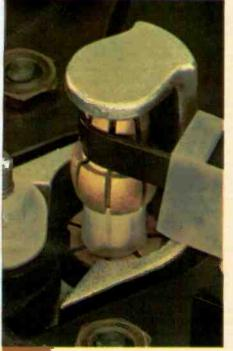
Motor pulley used in Dual's belt-drive models (1249, 601 and 510) is individually machined for perfect concentricity and balance. The drive belt is also precisionground to close tolerarces, contributing further to the smoothness of the drive system.
