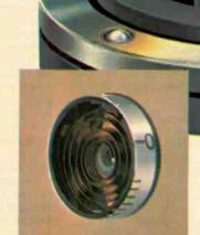
Stylus pressure is applied by long coiled spring, centered around vertical pivot. This system applies stylus pressure perpendicular to record and thus maintains the pressure equally on both groove walls even if turntable is not perfectly level
