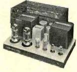
high-power triode vacuum tube for the amplifier's output stage and also created a new high-voltage tube for the driver section. In addition, the amplifier uses Luxman's quadrafilar-wound output transformer.
