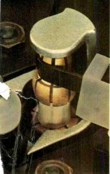
Motor pulley used in Dual's belt-drive models (1249, 601 and 510) is individually machined for perfect concentricity and balance. The drive belt is also precisiorground to close tolerances, contributing further to the smoothness of the drive system.
