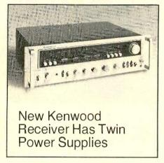
☐ At 160 watts per channel continuous into 8 ohms, 20 to 20,000 Hz, the Model KR-9600 is the top of Kenwood's present receiver line. Each of the two channels has its own completely separate power supply, ensuring fully independent operation. Harmonic and intermodulation distortion are both 0.08 per cent or less at rated output. Signal-to-noise ratios are 80 dB for the two phono inputs and 95 dB for the high-level inputs.
