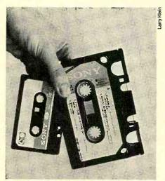
Photo illustrates relative sizes, if not the virtues, of the cassette and elcaset tape formats.
