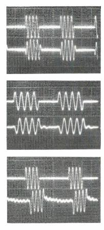
The Stereopillow's tone-burst response was quite faithful, as shown in these oscilloscope photos made at (top to bottom) 50, 500, and 5,000 Hz.
