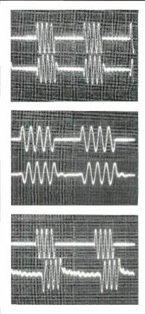
The Stereopillow's tone-burst response was quite faithful, as shown in these oscilloscope photos made at (top to bottom) 50, 500, and 5,000 Hz.
