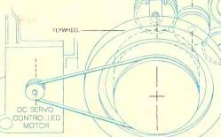
Tape Transport. In the CR5110 a large, dynamically-balanced heavy weight flywheel is driven by a regulated speed DC motor. The CR5115 uses servo control to provide even more precise tape speed. A precision-ground capstan provides good tape-to-head contact and accurate tape movement. Wow and flutter on the CR5110 is less than 0.09% WRMS; on the CR5115, less than 0.07% WRMS.
