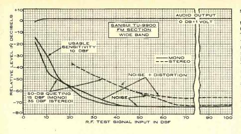
lectivity), with distortion ratings of 0.5 and 0.8 per cent, respectively, in mono and stereo. In the WIDE mode, the distortion ratings are dramatically improved to 0.06 and 0.08 per cent. Selectivity is reduced to 55 dB, which is adequate under most circumstances.
