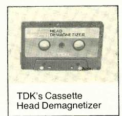
$\Box$  TDK has announced two new cassettedeck accessories, a head-cleaning kit and a head demagnetizer. The HD-1 demagnetizer (shown) is built into a standard compact-cassette case. It is inserted into the deck like a regular cassette and the deck is then set in the play mode; when a red LED on the demagnetizer lights up, the demagnetizing cycle is complete. The HD-1 is powered by a miniature 1.5-volt cell. Price: about \$20.
