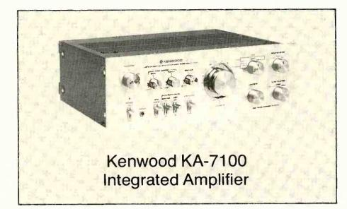
KENWOOD'S new KA-7100 integrated amplifier is a moderate-price product with outstandingly low distortion specifications and ample control flexibility for a wellequipped hi-fi system. It is rated to deliver 60 watts per channel to 8-ohm loads from 20 to 20.000 Hz, with less than 0.02 per cent total harmonic distortion. The KA-7100 has separate power supplies for its two channels, fed by a common power transformer. The poweramplifier sections of the KA-7100 are directcoupled.
