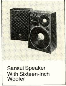
□ The SP-X9000 from Sansui is a new fourway bookshelf-size speaker system employing a 16-inch woofer in a bass-reflex enclosure. Other drivers include an 8-inch midrange, two horn tweeters with 6 x 2-inch mouths, and two  $1\frac{3}{4}$ -inch horn-loaded "super tweeters" with Mylar diaphragms. Crossover frequencies are 1,000, 6,000, and 10,000 Hz. The system has a three-position level control for the tweeters.
