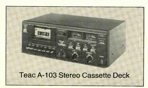
THE Teac A-103 is a moderately priced front-loading cassette deck with the darkgray and black appearance currently popular in audio-component styling. The tape transport, which occupies most of the left side of the unit, uses a single d.c. servo-controlled motor. The cassette itself loads into a slot in the door.
