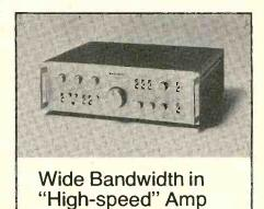
☐ The Kenwood KA-907 integrated amplifier uses the same basic circuit techniques that were employed in the design of Kenwood's esoteric series of single-channel amplifiers. The point of these techniques is said to be to reduce transient forms of distortion by increasing bandwidth (0 to 400 kHz for the Model 907) and improving the amplifier's reaction to complex, rapid waveforms.
