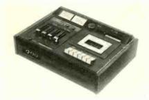
noise-reduction system; S/N 60 dB (with Dolby); wow & flutter 0.10% rms; has cue & review switch; tape-scan indicator; 3-digit tape counter; separate left/right channel slide level controls; two VU meters; separate left/right mike inputs; line-in terminals; headphone jacks.  $4^{*}$  H  $\times$  16" W  $\times$  11<sup>3</sup>/4" D ...... \$199.95
