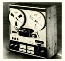
transport control, pause control with indicator light, dual VU meters; separate bias/equalization switches; separate mike/line inputs; separate mike/line level controls. Will handle up to 7" reels. Includes memory counter for automatic repeat and memory marker level guides; total remote-control capability. Response 40-24,000 Hz; wow & flutter 0.06% both at  $71/_2$  ips. S/N 65 dB (WTD at 3% THD).  $179/_{16}$  × 19¼<sup>"</sup> × 8½" ..... \$699.50
