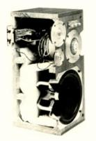
system; 12" woofer,  $2^{1}/_{2}$ " dome mid-range, 1" dome tweeter, 5/8" dome super tweeter; response 30-35,000 Hz; crossovers: ferrite core inductors 600, 5000, 10,000 Hz; metalized polyester film capacitors above 10,000 Hz; imp. 6 ohms; output acoustic pressure 90 dB/W at 1 meter; will handle 100 W peak.  $14^{1}/_{4}$ " W ×  $24^{1}/_{2}$ " H × 13" D ...... \$580.00
