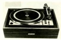
angle selector for single- and multiple-play. Tracking down to  $\frac{1}{2}$  gram. Damped counterbalance with coarse and fine adjustments. Synchronous/hi-torque motor, 4-lb one-piece die-cast platter; illuminated strobe.  $13'' \times 10^{3} \mu$ plus 1" at rear and right for tonearm overhang. 5" above and  $2^{3}\mu$ " below mounting board..... \$199.95
