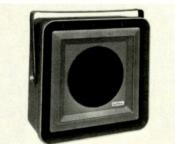
4000 Hz crossover; response 80-10,000 Hz; power handling 60 W peak; 8 ohms imp.; 120degree dispersion; compression-molded glassfilled polyester enclosure; water-proof & fungus-proof, 21<sup>1</sup>/<sub>2</sub>" H × 21<sup>1</sup>/<sub>2</sub>" W × 8<sup>1</sup>/<sub>2</sub>" D...... \$109.50
