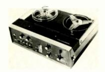
Portable (15 V, ten 11/2-V cells), mono design. Three speeds (71/2, 33/4, 17/8 ips), and has three heads. Will handle up to 7" reels. Has automatic level-input controls, mike & line mixing, and built-in speaker. Response 40-16,000 Hz ±2 dB at 71/2 ips, wow 0.1% at 71/2 ips, (S + N)/N 58 dB unweighted.  $13" \text{ W} \times 10" \text{ D} \times 4"$ .
