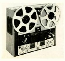
counter. Has full range of inputs and outputs. Response (record/piay) 30-17,000 Hz  $\pm 2$  dB at 7½ ips, 40-14,000 Hz  $\pm 3$  dB at 3¾ ips, 50-7000 Hz  $\pm 3$  dB at 1½ ips. Available in 2- and 4-track stereo models; with or without amplifiers and speakers; 15, 7½, 3¾ ips operation; optional Dolby-B noise reduction with every speed configuration........ \$1025 to \$1200
