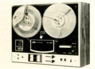
$7\frac{1}{2}$  ips; (S + N)/N -52 dB; wow & flutter 0.13% rms at  $7\frac{1}{2}$  ips. Has mike (0.5 mV) & aux. (80 mV) inputs. Line output 0-1 V. Has switch for either low-noise or standard tape; two heads (record/play and erase).  $7\frac{1}{2}\times 15\frac{1}{4}$  W × 124ar D. \$249.95
