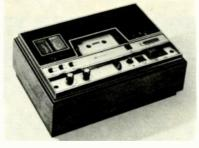
just Dolby system; a bias & equalizing switch for chromium-dioxide or standard tapes; VU meters; and mike inputs; response 40-14,000 Hz  $\pm$ 3 dB (CrO<sub>2</sub> tape); hum & noise -58 dB (with Dolby); wow & flutter 0.25% rms; dist. 0.2% (electronics only). Walnut-stained veneer base.
