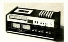
tion for various tape types; mike/line inputs (mixable); two separate erase and record/ playback heads. S/N 60 dB (with Dolby); wow & flutter 0.07%. Response 30-11,000 Hz with standard tape (30-15,000 Hz with own-noise tape; 30-16,000 Hz with chromium-dioxide tape). Inputs: mike 0.25 mV; line 0.1 V. Output: 0.3 V. 7" H  $\times$  17<sup>1</sup>/<sub>2</sub>" W  $\times$  10<sup>5</sup>/<sub>8</sub>"...... \$479.50
