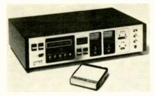
3M ferric-oxide tape. Has minutes/seconds timer for precise timing of recordings; fastforward mode 31/2 times actual speed; special cueing system. Response 30-15,000 Hz ±3 dB with Scotch special high-performance tape (30-12,000 Hz with standard tape). (S+N)/N 60 dB at 4000 Hz and above (Dolby system on). Sensitivity: mike 0.25 mV; aux. 80 mV. 193/4" × 5" × 10¼".....\$399.95
