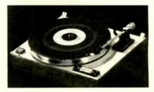
drive; viscous-damped cueing control; wow & flutter 0.017% (DIN 45507 weighted); rumble -60 dB (DIN 45539 weighted); stylus force range 0-4 gr; tracking error  $\pm 1.7$  degrees max; adjustable anti-skate with separate scales for all types of styli. Comes with dust cover, walnut base, cartridge, low-capacity tonearm, extension cord cables.  $13'' \times 14^{3}/4'' \times 7''$  D.
