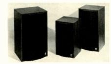
heavy-duty woofer, Biconex horn/compression driver mid-range, and dome super tweeter. Max. rms amplifier power 75 W/ch. Response 30-23,000 Hz. Has a continuously variable tonalbalance control and an automatic dynamic tonal balance control with defeat switch. Dispersion 120° × 120°. Has removable reticulated foam grille available in black, brown, burnt orange, or blue.  $194_4^{\prime\prime} \times 12^{\prime\prime} \times 11^{1}2^{\prime\prime}$  D...... \$119.50
