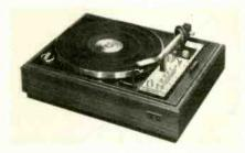
control; synchronous motor; direct-drive; record repeat, cueing & pitch controls; stylus wear indicator; accessory tray; stylus pressure adjustable from 0 to 4 g; 7¼-1b platter; removable cartridge shell; comes with walnut base, dust cover, and Shure M-91ED magnetic cartridge \$299.80
