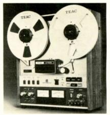
Two-speed (15 & 71/2 ips), two-track, two-channel stereo with four heads (erase, record, playback, 4-track playback); 3 motors. Will handle 101/2" & 7" reels. Features cue button & flip-up head cover for easy editing; auto stop counter; mike attenuation control; LED peak level indicators. Response 30-26,000 Hz at 15 ips; wow & flutter 0.04% at 15 ips; S/N 67 dB (WTD at 3% THD). 17%  $^{\prime\prime}$  W  $\times$  20½  $^{\prime\prime}$  H  $\times$  8¼  $^{\prime\prime}$  D. . \$1049.50
