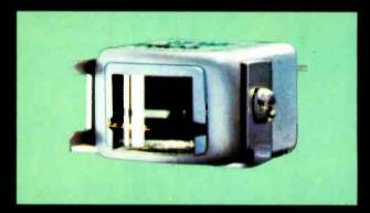
recorders. As a result, the heads wear much longer and you're unlikely to encounter reduced high-frequency response due to a widening playback gap.
