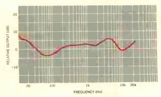
Fig. 3. Only an equalizer, not tone controls, could achieve this curve.
