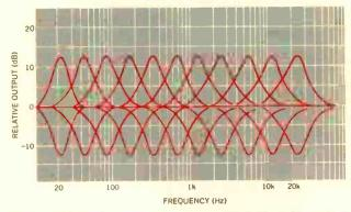
Fig. 2. Each equalizer control boosts or cuts part of the audio spectrum.
