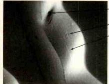
Pit from dust abrasion.Ground-in microdust.Prominent dust abrasion.
