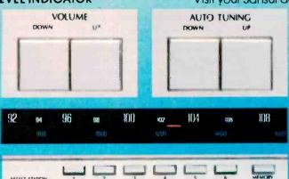
to 12 user-selected stations may be "stored" in the 5900Z's memory circuits for instant recall. The last station received will be remembered when the tuner is turned on again; and memories are kept "live" even during a power outage.
