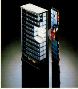
A cutaway of the Matrix 2 from England's B&W Loudspeakers shows the extremely rigid, cellular honeycomb structure of its cross members. Matrix series speakers are designed for minimal, fast-decaying cabinet radiation to avoid coloring the drivers' output.
