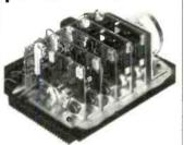
With these high standards, all components—not just the signal correction circuitry—incorporate the most sophisticated technical advances. The entire system reflects the design approach customary in industrial electronics like using thick film modules with SMD's (Surface Mounted Devices), bus interface connections, and plug-in card technology for high reliability and performance capability.
