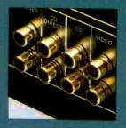
Gold-plated input jacks on the Citation twentyone preamplifier provide reduced signal loss and improved longterm conductivity
