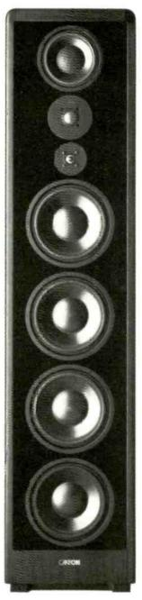
The top-of-the line CA 30 active speaker is a 4-way system powered by 7 internal ampilifiers (ane for each driver). The woofers are powered by 4x120 Watt amplifiers, the midranges by 2x100 Watt amplifiers and the titanium tweeter by 1x100 Watt amplifier. A total of 780 Watts per CA 30 soeaker. In addition, problems normaily associated with passive crossover networks are non-existent due to Canton's advanced MOS-FET electronic crossovers.
