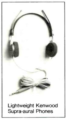
□ Kenwood's KH-7, KH-5 (shown), and KH-3 stereo headphones are supra-aural types designed to produce a sound-pressure response tailored appropriately for human hearing. All three have pressure-molded polyester diaphragms about 1 inch in diameter and lightweight rare-earth magnets to give high power capability and low distortion. Each headphone set comes with an extra pair of snap-off foam ear cushions and a comfortable headband.
