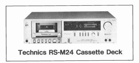
THE Technics RS-M24 is a front-loading, two-head cassette deck that employs a single-capstan, single-d.c.-motor drive system. The record/playback head is made of "MX" permalloy, which is capable of accepting the very high bias current required by metal-alloy tape. The transport controls, though mechanical, utilize soft-touch pushbuttons that provide much of the feel and flexibility normally associated with sole noidoperated controls.
